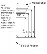
Figure 9 - Minimum Mantel Clearances for Built-In Installation
